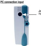
Jack connector (3.5) Input for KISTOCK-PC software
